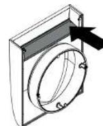
Once all work inside the building has been completed, the inside cover can be installed. Place the filter unit in the slots for the filter inside the cover. Insert the cover into the mounting tube, making sure that the air vent points upwards and that the cover sits tightly.
