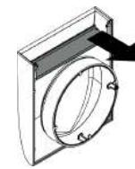
Step 2: Pull the flap out of the flexible foam.
