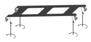
3. Support the fan in the support guides and fix the screws to secure the unit to the support.
