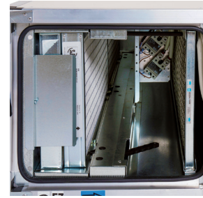
Easy access to filters through panels, side or bottom. Two filtering options: - Long version P F7 with capacity for mounting two filters: F7 with very low built-in pressure drop and possibility of mounting a second filter (supplied as an accessory). The filter clamping system with articulated arms ensures excellent sealing of the filter assembly. - M5 short version with capacity to allow a single M5 filter mounted over a rail without filter clamping devices.
