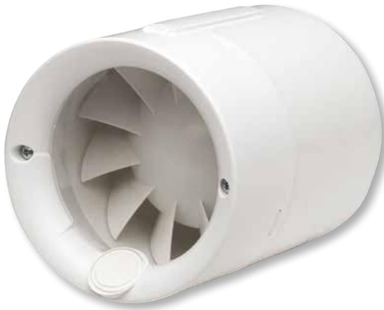
Transfer axial fan offering a very low noise level and specifically designed to work through a duct or to be flush mounted into the wall, ideal for ventilating small areas or to exchange heat between adjoining rooms. Fitted with single phase motors 230V-50Hz, IP44, Class II, with ball bearings for enhanced working life and assembled on silent-blocks.
