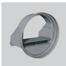
RD BP SM Auto-adjustable flow regulators. To be installed inside the cuff of the BDOP nozzles. 80mm diameter. Flow rate: 15 or 30 m³/h.
