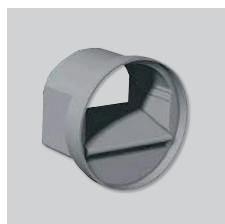
RD BP Auto-adjustable low-pressure flow regulators. (20-100 PA) To be installed inside the duct. 80mm diameter. Flow rate: 15 or 30 m³/h.
