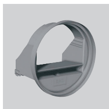
RD BP SM Specific low-pressure (20-100 Pa) and self-adjusting damper without sleeve to fit directly into the sleeve of the BDOP. 80mm diameter. Airflow: 15 or 30 m³/h.
