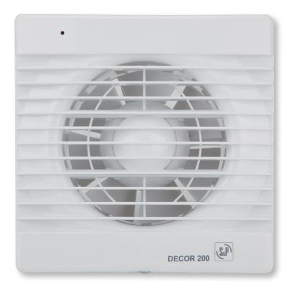
Range of axial extractors with airflow rates of 180 m<sup>3</sup>/h, for connection to 120 mm diameter circular ducting. All the fans are manufactured from injection moulded plastic, fitted with neon light indicator and single phase 230V-50Hz, class B motor equipped with overload thermal protection. The "Z" versions incorporate long life motors fitted with ball bearings. All the fans are class II insulation, IPX4 rated and suitable to operate with air temperature up to 40°C.
