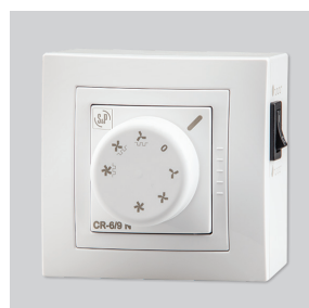
CR-6/9 N 2 Power selector and 3 speed remote fitted with the fan to control up to 5 units in series of the A/H models (ambient and hot air) . LxWxH (mm): 88x47x88
