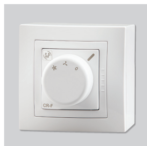
CR-F 2 Power selector remote fitted with the fan to control up to 5 units in series of the A models (only ambient air) . LxWxH (mm): 88x47x88
