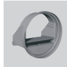
RD BP SM Specific low-pressure (20-100 Pa) and self-adjusting damper without sleeve to fit directly into the sleeve of the BDOP. 80mm diameter. Airflow: 15 or 30 m 3 /h.
